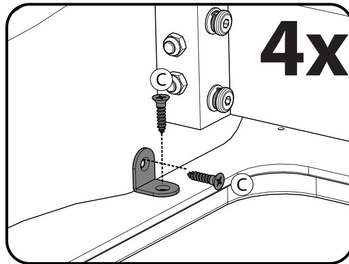
! Partially tighten screws. Once all have been installed, fully tighten all screws
