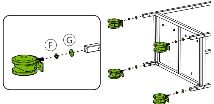
**!** Note: Return cart to upright position once casters are installed. Check casters every 6 months and tighten as needed.
