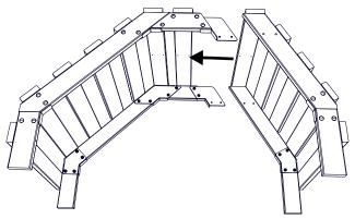
Hammer the bolts into the pre-drilled holes until they cannot turn.
