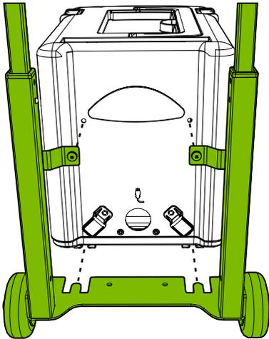
2 Fasten Hardware Through Inside of Tech Tub
